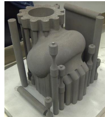
Fuel Turbine Bypass Valve
