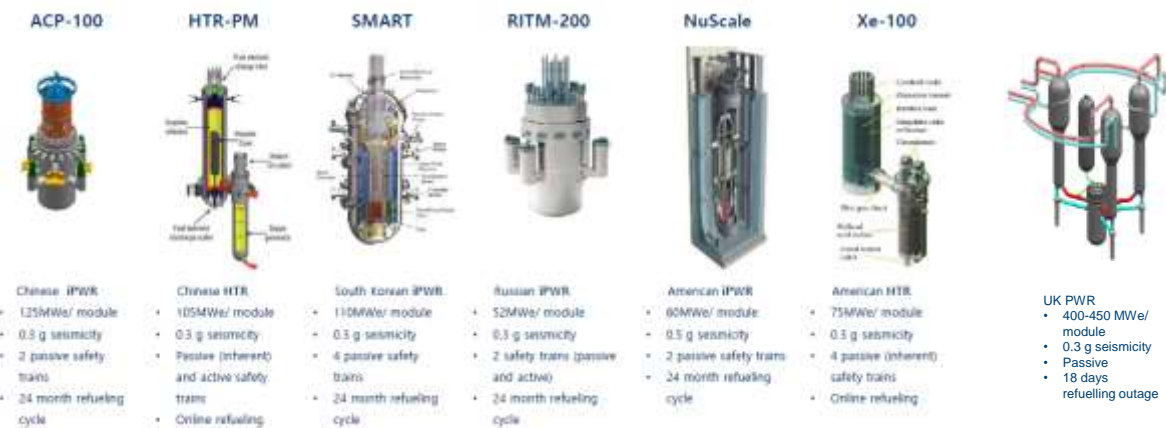
Figure 3: Examples of international SMR designs
