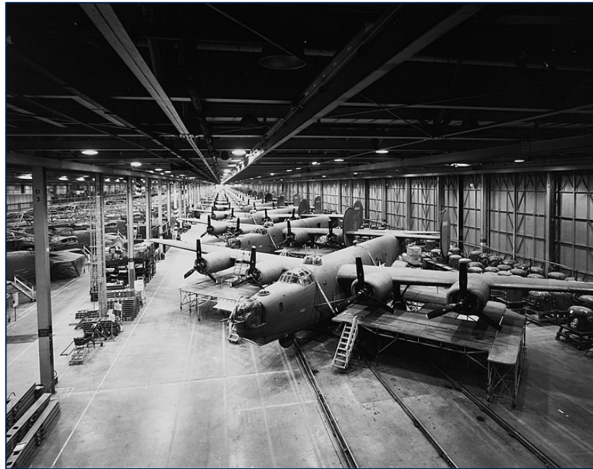
B-24 Final Assembly, San Diego, California
