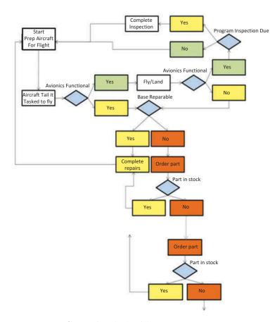
FIGURE 1 Avionics failure test process.
