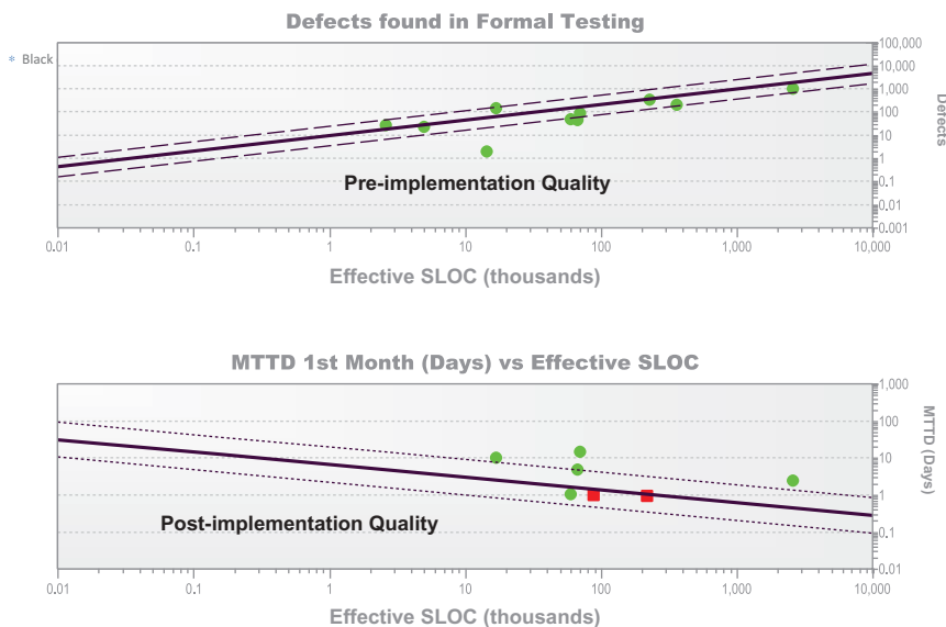
FIGURE 3 Defects during Formal Testing vs. Effective SLOC and MTTD 1st month vs. Effective SLOC.
