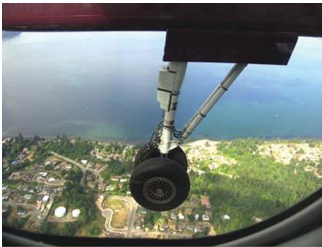
FIGURE 1 Fully extended MLG of a Q400 (color figure available online).
