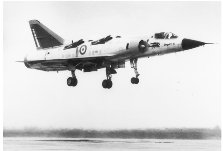
Dassault Mirage IIIV vertical take-off and landing aircraft. Two prototypes were developed in 1965 and 1966, but the project was abandoned shortly after one crashed. The number of engineers and draftsmen on the project peaked at 30.
