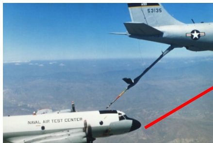
Universal Aerial Refueling Receptacle Slipway Installation
