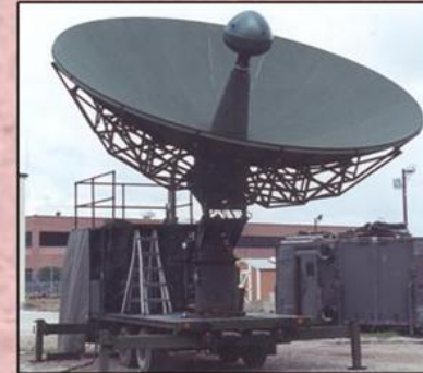
Primary Predator Satellite Link (SATCOM / Beyond Line of Sight)
