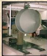
Ground Data Terminal (Line of Sight Link)
