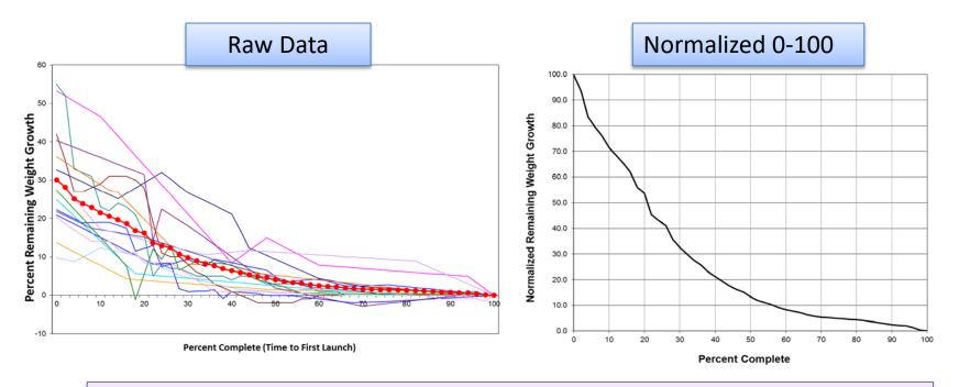
Normalized curve used for CAAG estimates during program execution Unit-level WG model X Depletion Model = Estimated WG
