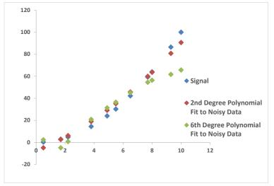
• Simpler polynomial is a better representation of the underlying signal – closer fit on 10 of 11 data points, and Pearson's R2 between actuals and estimates is 98% for simpler fit vs. 88% for the sixth-degree polynomial
