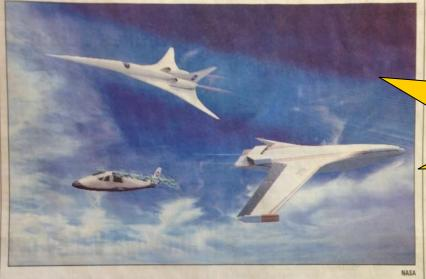
BEYOND TRADITIONAL - NASA's proposed 2017 budget the Antelope Valley. At top is a low sonic boom flight demonstrator, at contains money for three types of experimental aircraft to be tested in right is a hybrid wing body and at lower left is a hybrid electric aircraft.
