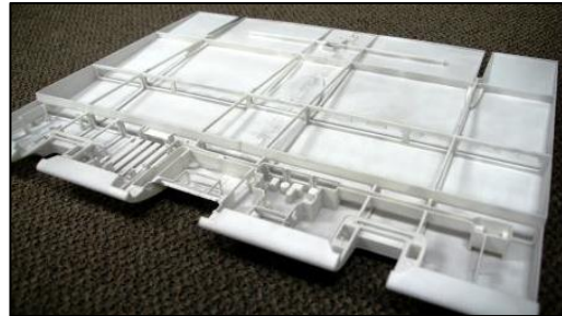
Figure 5 - Additively manufactured wing assembly
