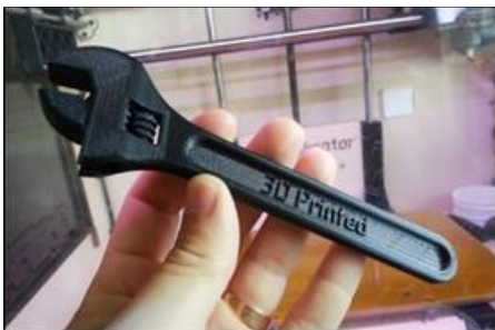
Figure 4 - Additively manufactured hand tool
