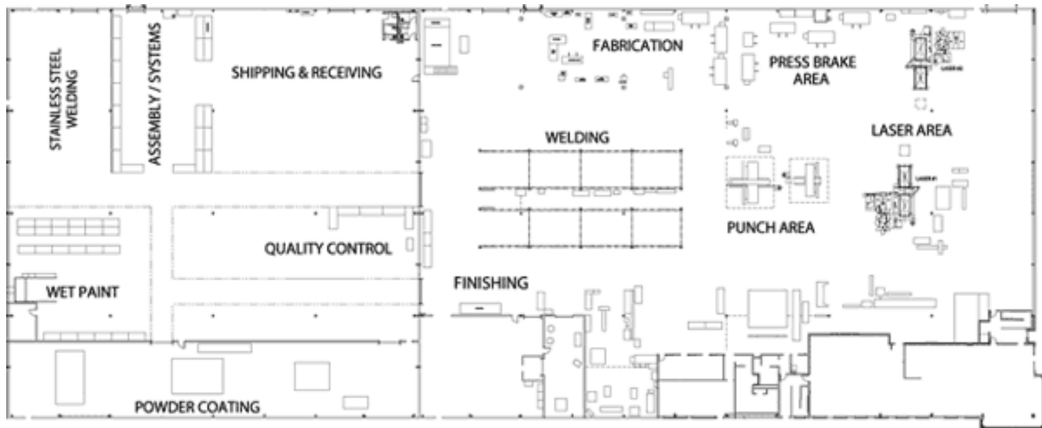
Figure: TruCut Fabricator Plant Layout
