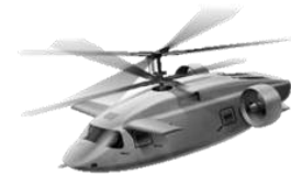
Concept 4: Coax compound /w ducted fan
